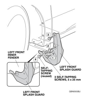
5. While holding the left front splash guard against the left front inner fender, tighten the four self-tapping screws in the order shown.
