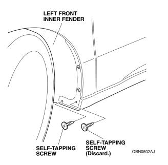
4. Loosely secure the left front splash guard on the left front inner fender with three 5 x 25 mm self-tapping screws provided and one self-tapping screw removed in step 3.
