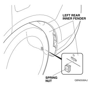
12. Loosely install the left rear splash guard to the left bracket and left rear inner fender with one 5 x 20 mm self-tapping screw provided and two self-tapping screws removed in step 7.
